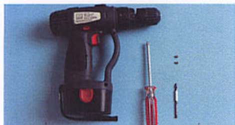
a1. Fitting tools required include Ø4mm drill bit, star point screwdriver
